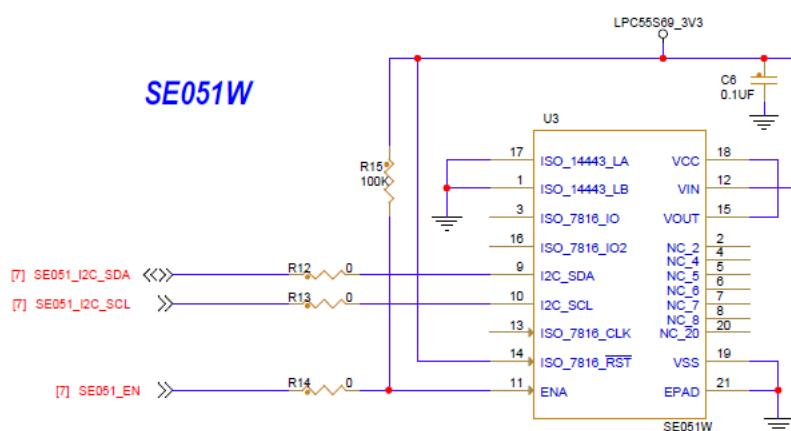
Figure 38. SE051W security element on the FACECV board
