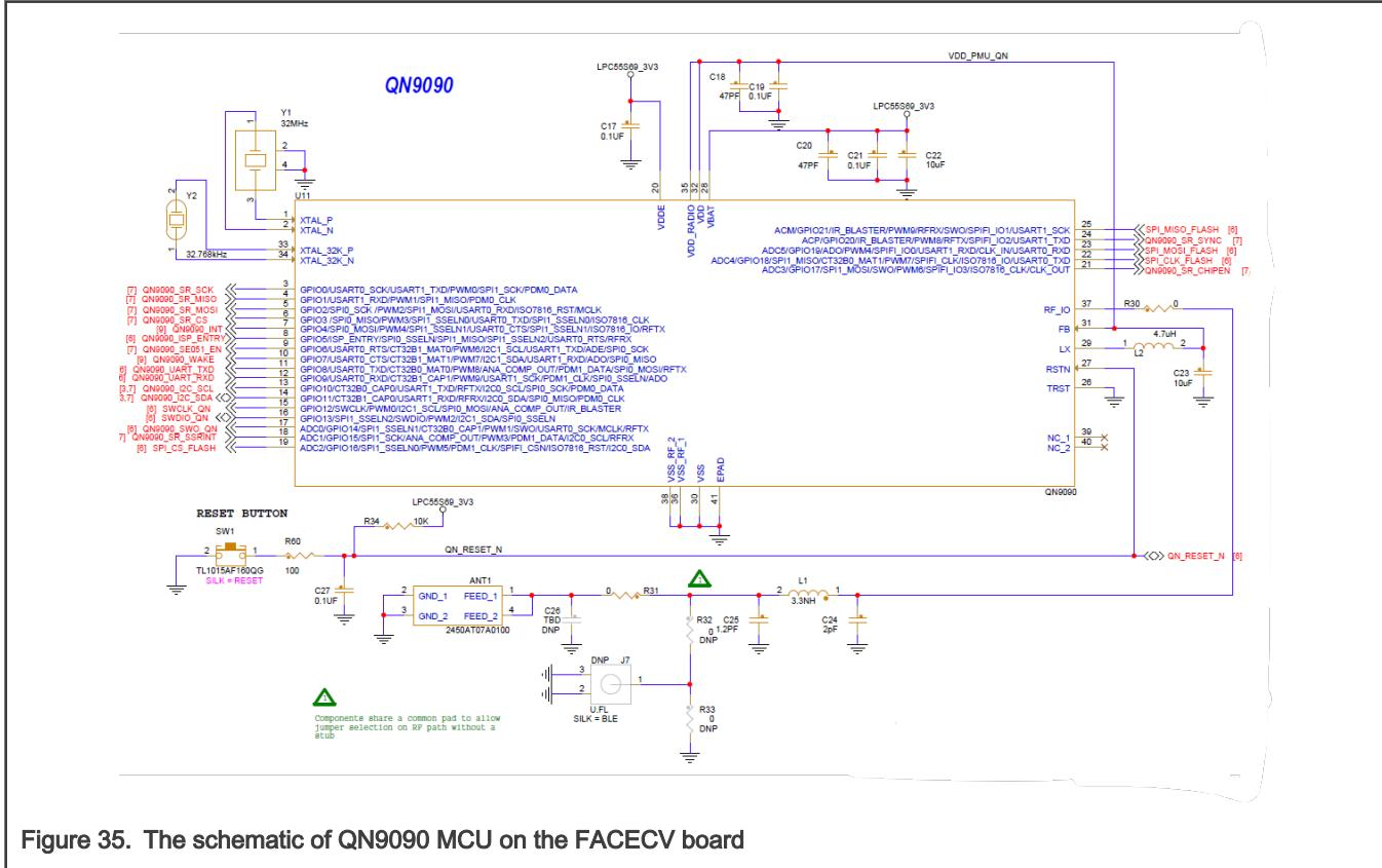
Figure 35. The schematic of QN9090 MCU on the FACECV board
