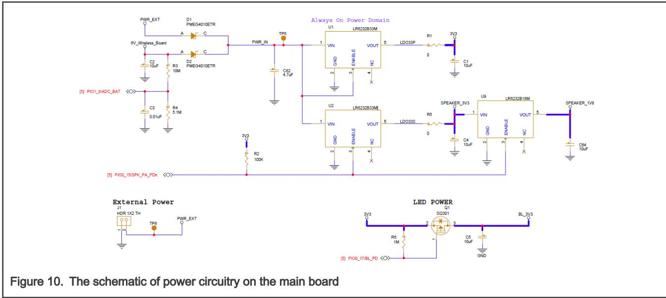
Figure 10. The schematic of power circuitry on the main board
