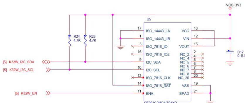
Figure 22. SE051H security element on the wireless board
