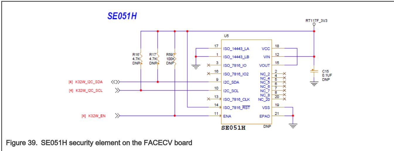
Figure 39. SE051H security element on the FACECV board
