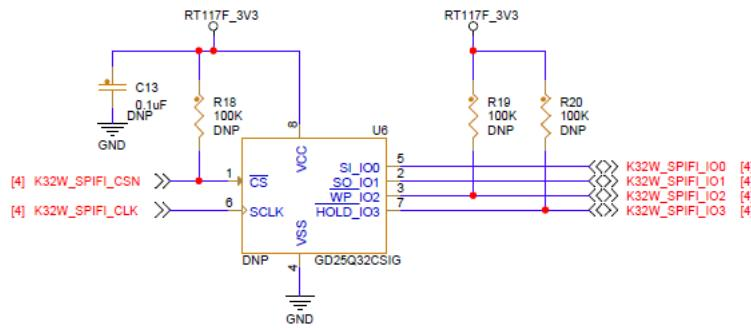
Figure 36. GD25Q32CSIG SPI NOR flash on the FACECV board
