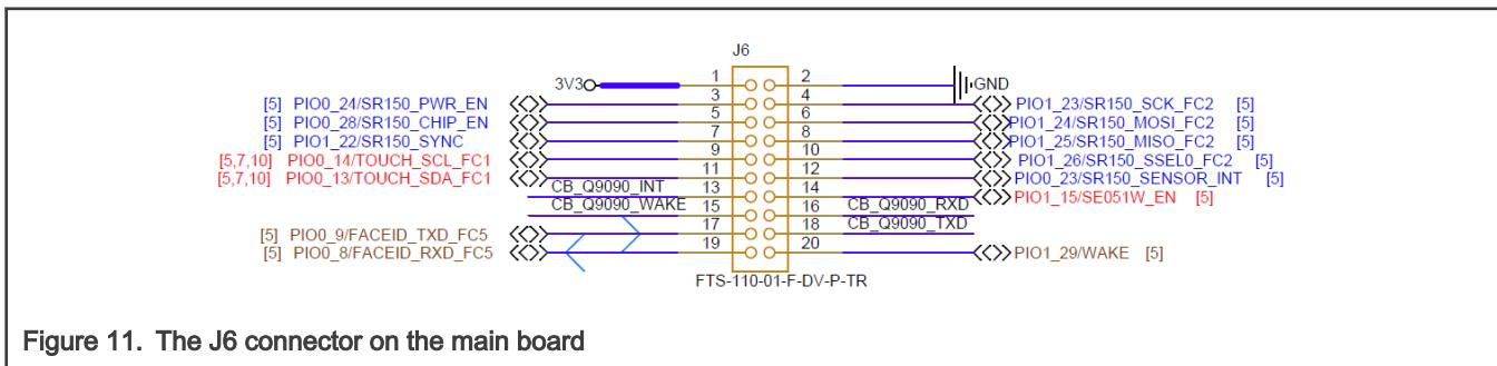
Figure 11. The J6 connector on the main board
