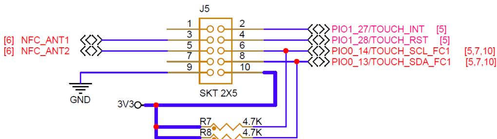
Figure 12. The J5 connector on the main board
