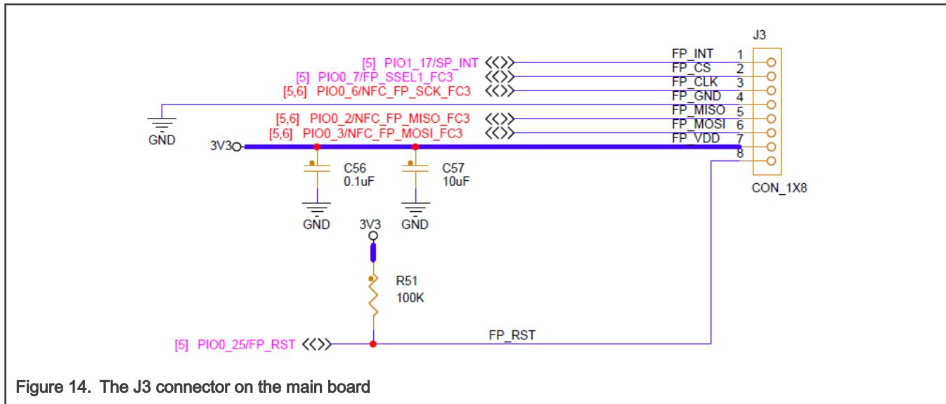
Table 11. The J3 connector pin allocation in the main board
