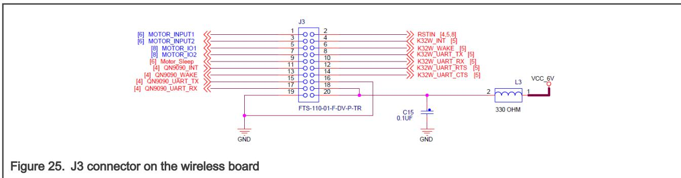
Figure 25. J3 connector on the wireless board
