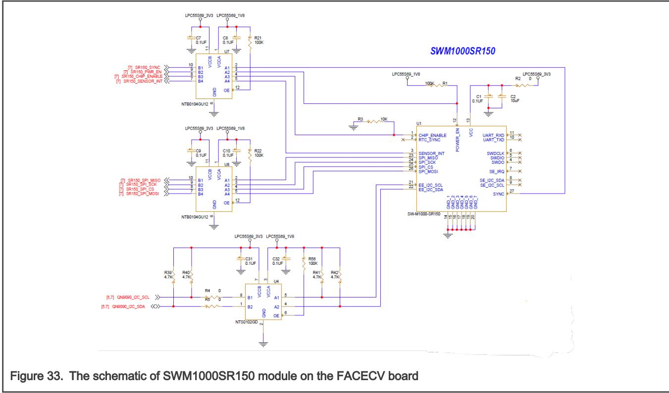
Figure 33. The schematic of SWM1000SR150 module on the FACECV board
