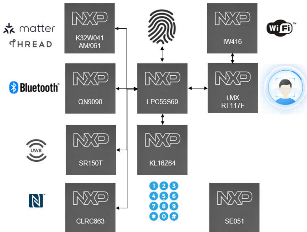
Figure 1. The main functions and modules of the Smart Access platform
