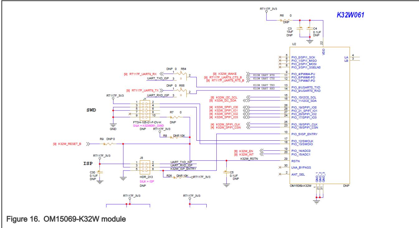
A pushbutton is connected to the RSTIN pin (reset input) of the OM15069-K32W module.
