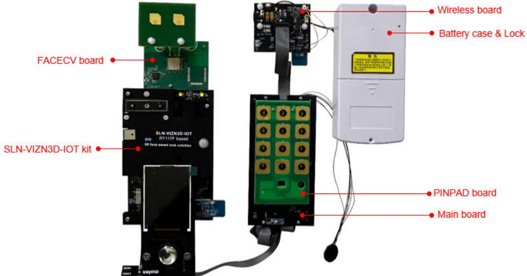
Figure 2. The Smart Access platform
