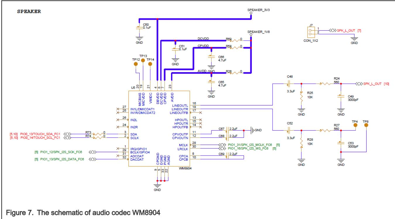
Figure 7. The schematic of audio codec WM8904
