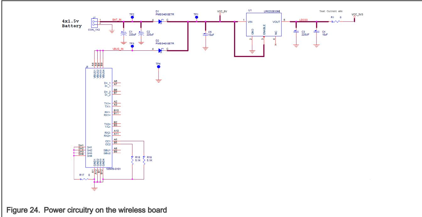
Figure 24. Power circuitry on the wireless board
