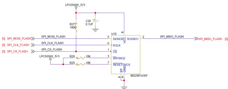
Figure 37. MX25R1635F SPI NOR flash on the FACECV board
